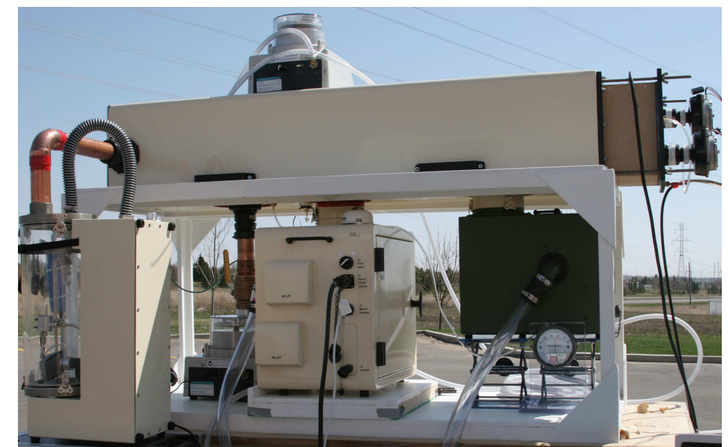
Figure 4. A typical outdoor setup of the CATS, Aerosol Diluter and equipment under test.
