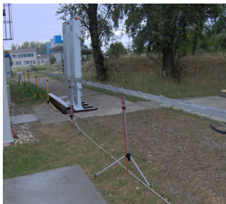
Source transport system for testing of portal monitors.
